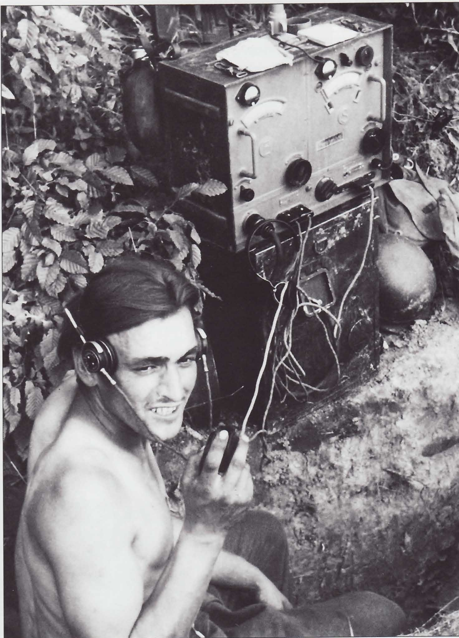
This Tornisterfunkgerät has been set-up on the edge of a slit trench sitting on the power supply and accessory case. The right half is the transmitter and the left is the receiver. The carrying cases were field gray (dark green), but were sometimes painted a green, brown, and sand camouflage pattern. The radio's front panels were field gray with the labeled plates light green with black markings. With voice it had about a six-mile range and 12 miles using continuous wave (Morse code).
