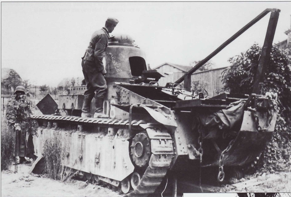
An abandoned Renault Char D1 heavy tank is inspected by two German NCOs. This tank, produced in only small numbers (160), was armed with a short 47mm gun and two 7.5mm machine guns. It had a three-man crew. The triangular framework on the right rear deck is the radio antenna. The assembly fitted to the tank's rear is to assist it when crossing ditches and gullies.
