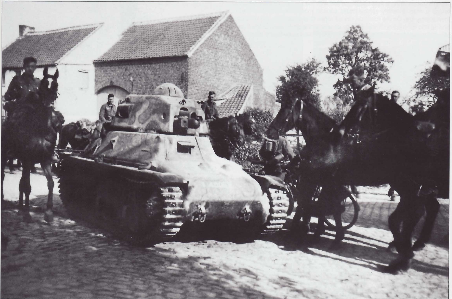
German mounted troops examine an abandoned Hotchkiss H39 tank. It was armed with a 37mm gun and a 7.5mm machine gun. This light tank was manned by a two-man crew. The Germans pressed these into service as the PzKpfw 38H(f) mainly assigning them to security and coastal defense units in occupied countries. Other models of captured French tanks were employed in the same manner.
