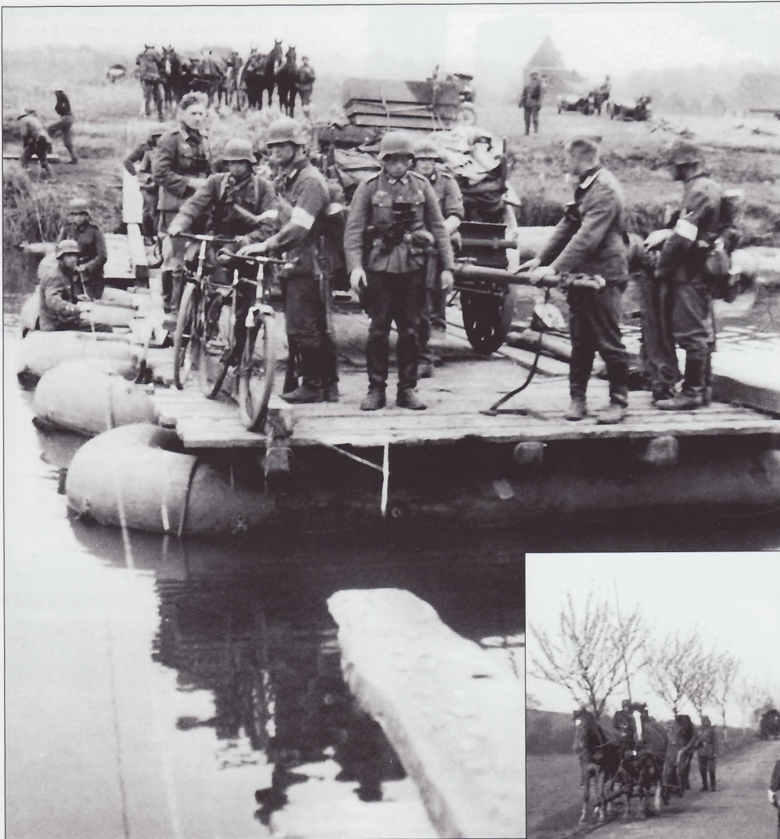
An artillery caisson is floated across a narrow river on a larger pontoon ferry using four six-meter medium pneumatic boats. They could be configured as 2.25-ton (two boats), 4.5-ton (four boats), and 9-ton ferries (six boats in tandem).
