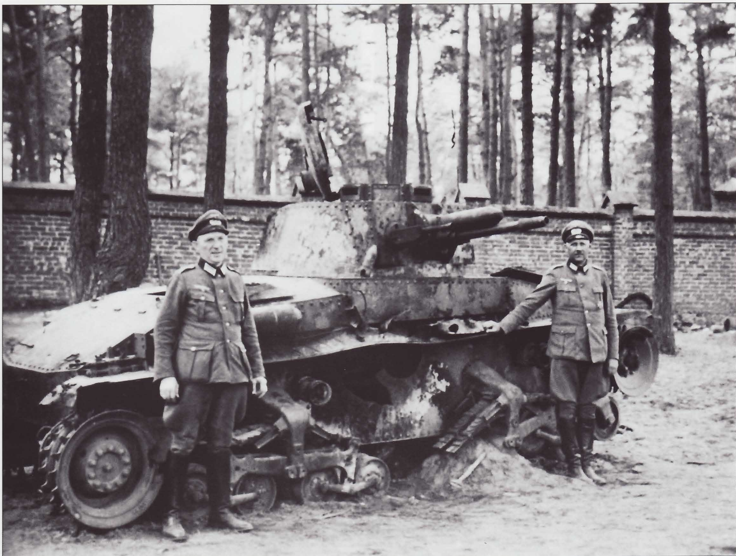
Two Wehrmachtsbeamte (Defense Forces officials) inspect a burned out PzKpfw 35(t) tank. This was a former Czechoslovak Lt vz35 employed by the Germans. It was armed with a 3.7cm gun and two 7.92mm vz37 machine guns, redesignated by the Germans as the MG37(t). Some 220 were taken into German service with most assigned to 6.Panzer-Division. They campaigned in Poland, France, and Russia until withdrawn from frontline service in 1942 and most survivors were converted to self-propelled guns.
