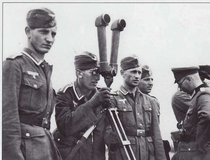
A group of Unteroffizieren survey a forward area using a 6x30 Sf.14Z scissors periscope (Scherenfernrohr). It is obvious why soldiers nicknamed it the Eselsohren (donkey ears). These are possibly gun commanders of an artillery battery.
