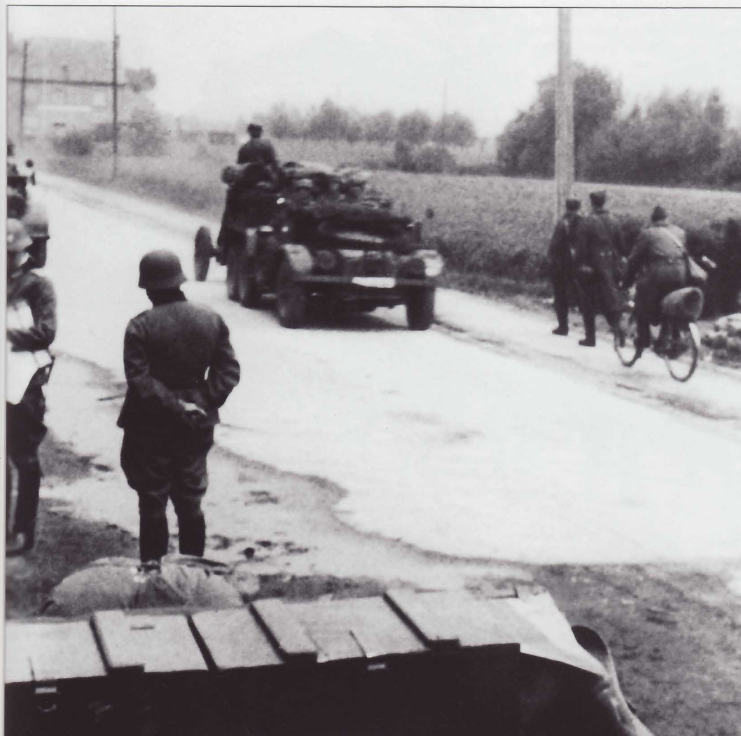
A Krupp-Protze LKW Kfz 69 truck tows a 3.7mm PaK 35/37 antitank gun. Protze translates to "limber." Another version, the Kfz 81, towed the 2cm anti-aircraft gun.
